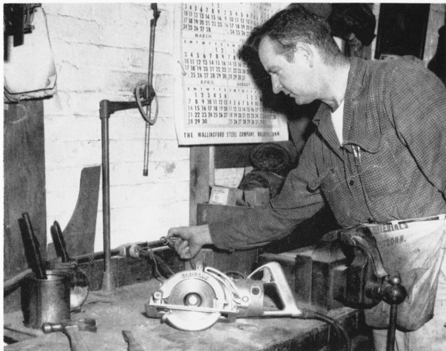
Edward Venslovas, Carpenter Shop, guards against possible electrical shock by using the "third wire" to ground an electric saw—before using it.
